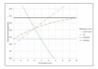
With the perturbation ranges and probability distributions defined, we can now look at the tolerances associated with an entire production run. To do this, we performed a Monte Carlo tolerance analysis, during which a large number of trials with randomly perturbed parameters was simulated. We ran 10,000 iterations for our analysis and looked at the statistics associated with each of our performance metrics.
